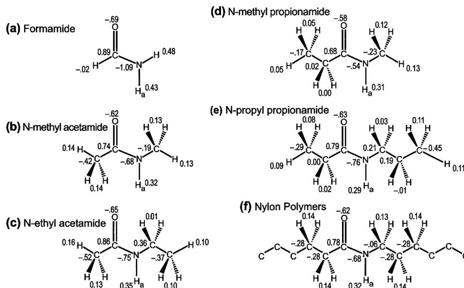
**Figure 6.** Charges for various amide models and nylon polymers.
