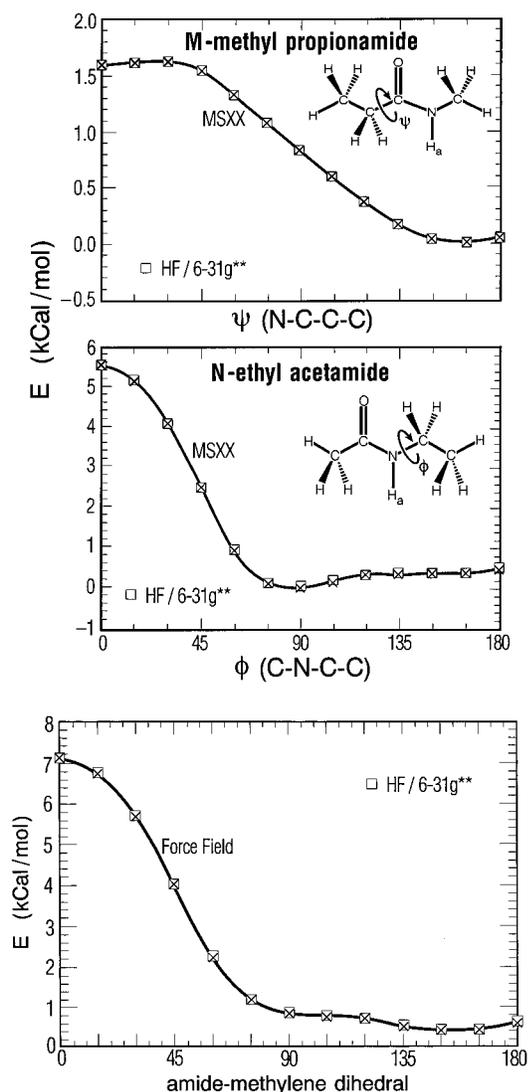
**Figure 5.** Torsional potentials: (a, top) the N(amide)–C(amide)–C–C dihedral in *N*-methylpropionamide, (b, middle) the C(amide)–N(amide)–C–C dihedral in *N*-ethylacetamide, (c, bottom) combination of both dihedrals. In each case the structure of the molecule was completely optimized for each value of the dihedral. Shown are the calculated values from HF/6-31G\*\* (□) and from the FF (× inside □). A smooth line is drawn through the FF points to guide the eye.
